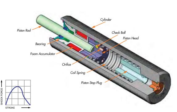
**Constant orifice area damping** (dashpot) provides the largest shock force at the beginning of the stroke when impact velocity is highest. These shock absorbers provide high-energy absorption in a small, economical design.
