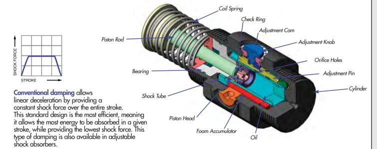
The adjustable multiple orifice shock absorber is similar to the principles described earlier. The check ring replaces the check ball and the adjustment feature uses an adjustment pin instead of an adjustment ball. The damping force of the shock absorber can be changed by turning the adjustment knob. Maximum damping force is achieved by turning the adjustment knob to eight (8), while minimum damping force is achieved by turning the adjustment knob to zero (0).
