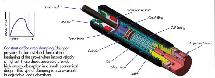
The damping force of an ITT Enidine single orifice shock absorber can be changed by turning the adjustment knob. Maximum damping force is achieved by turning the adjustment knob to eight (8), while minimum damping force is achieved by turning the adjustment knob to zero (0). Turning the adjustment knob causes the adjustment ball to increase or decrease the clearance (orifice area) between the ball and its seat, depending on rotation direction.
